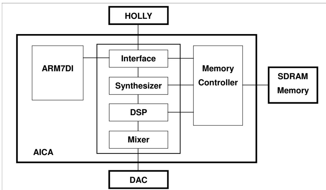
Figure 4-2 block diagram of the interior of AICA
