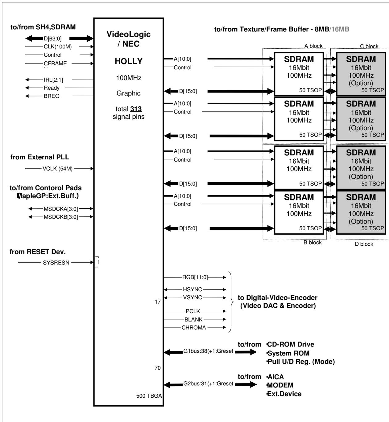
Figure 3-1 Block diagram of the HOLLY sub system
